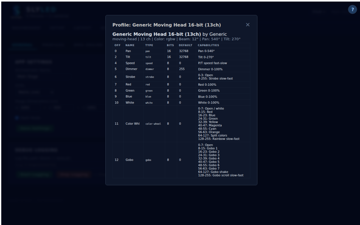
Moving Head 16-bit profile with 13 channels and capability ranges
